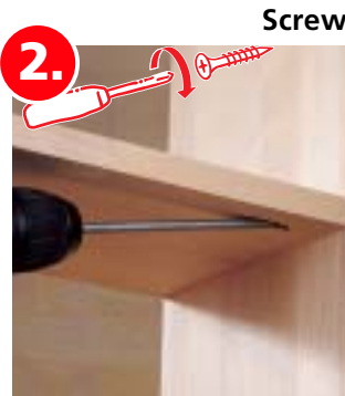
...you then join the two workpieces with wood screws...
