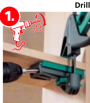
With the "Undercover Jig", you drill precise holes in the workpiece...
